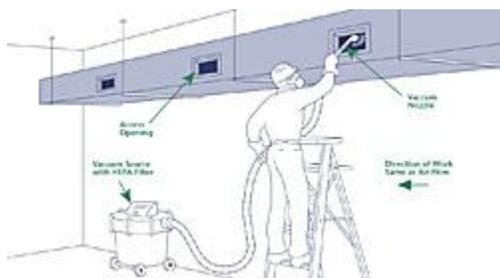
This method involves the use of a portable vacuum with High Efficiency Particulate Air (HEPA) filtration. There is direct contact between the brush head and the interior of duct surfaces to dislodge and remove dirt and debris.
